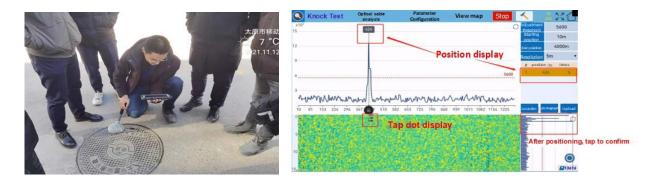
• Obtain the latitude and longitude information of the knocking point in real time and synchronize with GIS map together with the picture of the knocking point
