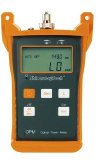
OPM-15 series Optical Power Meter paired with ShinewayTech SLS series Stabilized Laser Source can meet general test requirements of fiber identification, attenuation/loss measurements, continuity verification and transmission quality evaluation on singlemode and multimode fibers in LAN/WAN/CATV infrastructure. OPM-15 is ideal for both lab and field applications offering high quality, high stability and competitive low costs.
