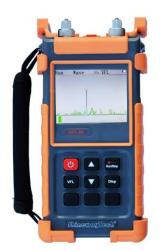
OFI-50A uses an optical fiber sensing principle to confirm the target fiber; It can quickly identify deep buried, overhead and pipe fiber cable without any destruction, and provides a simple identification method for maintenance personnel. Users only need to gently knock on cable, when knocking on the target cable, OFI-50 can clearly hear the knock on an earphone, which can accurately identify the target cable.
