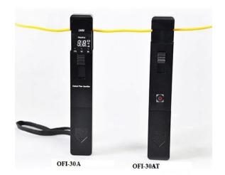
OFI-30A/AT can detect optical signals presence, type and direction anywhere on fibers during an optical network deployment, maintenance or troubleshooting. With non-destructive macro-bend detection technology, it introduces no damage to tested fiber or interference to the service on fiber.
