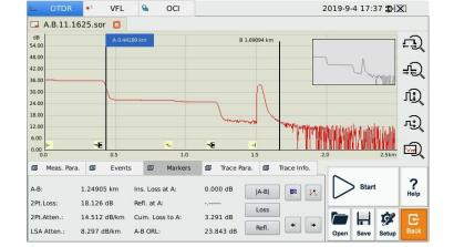
Fault locating, fiber length / loss / return loss measurement, connector / splice / splitter / macro bend / fiber-end detection
