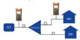
• Testing through splitter, splitter and fiber end identifiable
